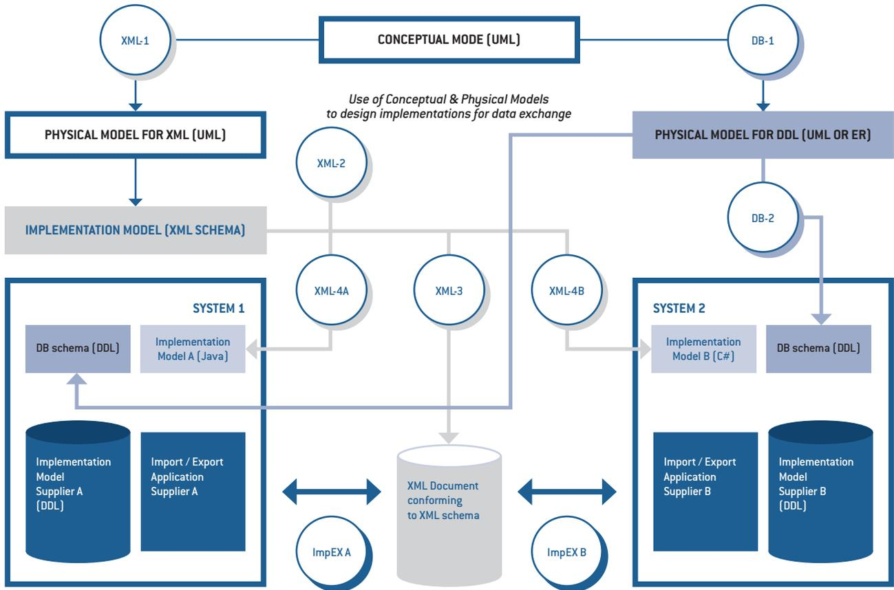
Figure 1 –Use of conceptual and physical models
